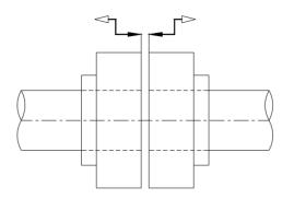
h2-By fitting couplings be sure that there is no exantricity between the two shafts.
