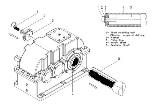
e2 -Use the disassemble set from YILMAZ and fasten the bold as shown bellow to take out the output shaft.
