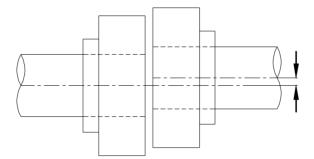
h3-By fitting couplings be sure that the two shafts are not angular miss-aligned.
